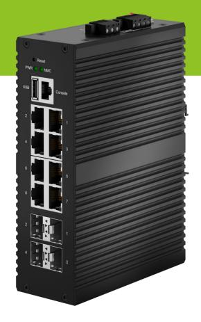
The industrial Ethernet switches are designed for use in harsh environments and allow you to build cost-effective, reliable, secure industrial networks. Whether you require an unmanaged switch for a point to point link, a managed switch for redundancy, our extensive range of industrial Ethernet switches and knowledge of the various standards used in train, railway, energy, utilities and road applications means we have the ideal solution, regardless of the environment.
