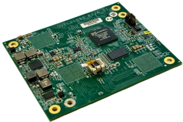
IronMan® Network Module MO-P8Cx-4F 8x1+4x10 (50 Gbps) MO-16Cx-4F 16x1+4x10 (72 Gbps) MO-24Cx-6F 24x1+6x10 (86 Gbps) MO-48Cx-6F 48x1+6x10 (110Gbps) MO-24Cx-28F 24x1+24x2.5+4x10 MO-13F 13x10 (132Gbps)
